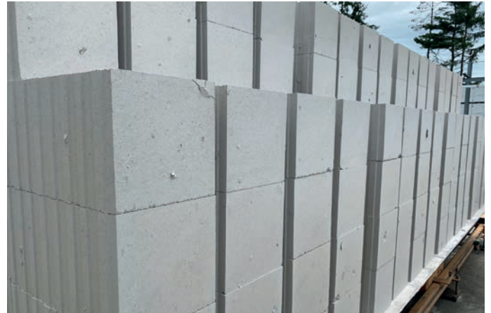
Figure 9: Calcium silicate masonry units made with BOF-1 before (left) and after (right) the autoclaving process in the technical scale test No. 2
