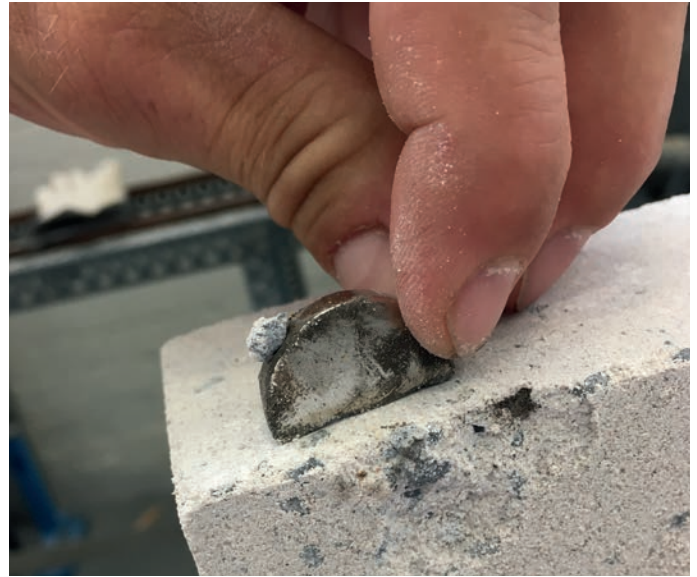
Figure 14: Magnetic BOF-1 grain from a damaged calcium silicate masonry unit made on a semi-technical scale
