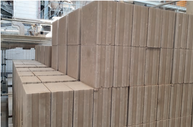
Figure 9: Calcium silicate masonry units made with BOF-1 before (left) and after (right) the autoclaving process in the technical scale test No. 2
