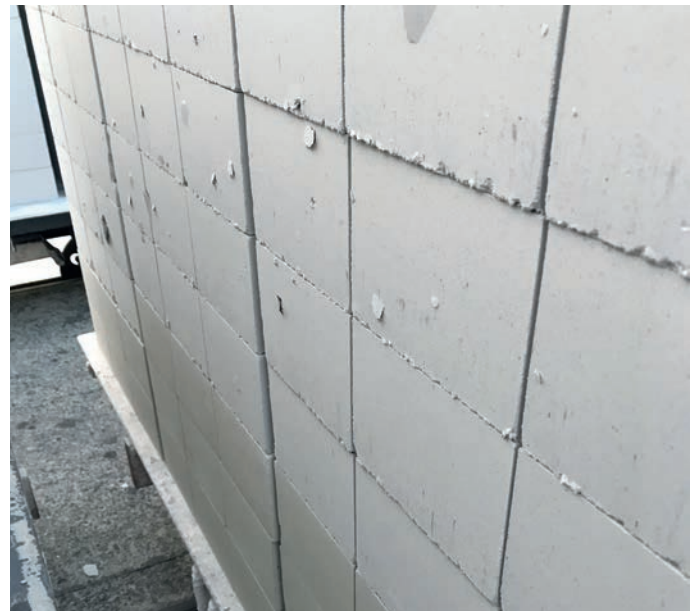
Figure 11: Calcium silicate masonry units made with EAF-1 after the technical scale test No. 1
