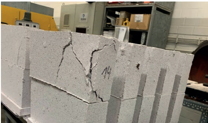
Figure 15: Damaged calcium silicate masonry units with 10 wt% BOF-2 made on a semi-technical scale
