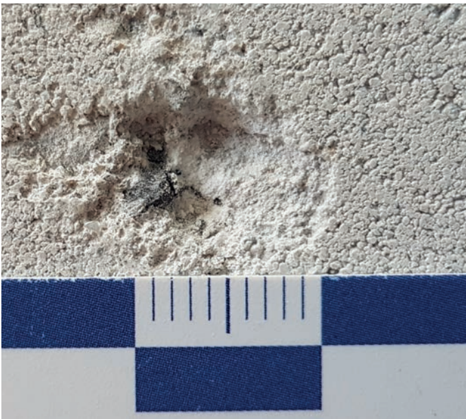
Figure 10: Damaged spot of a calcium silicate masonry unit made with 43 wt% BOF-1 after the technical scale test No. 2
