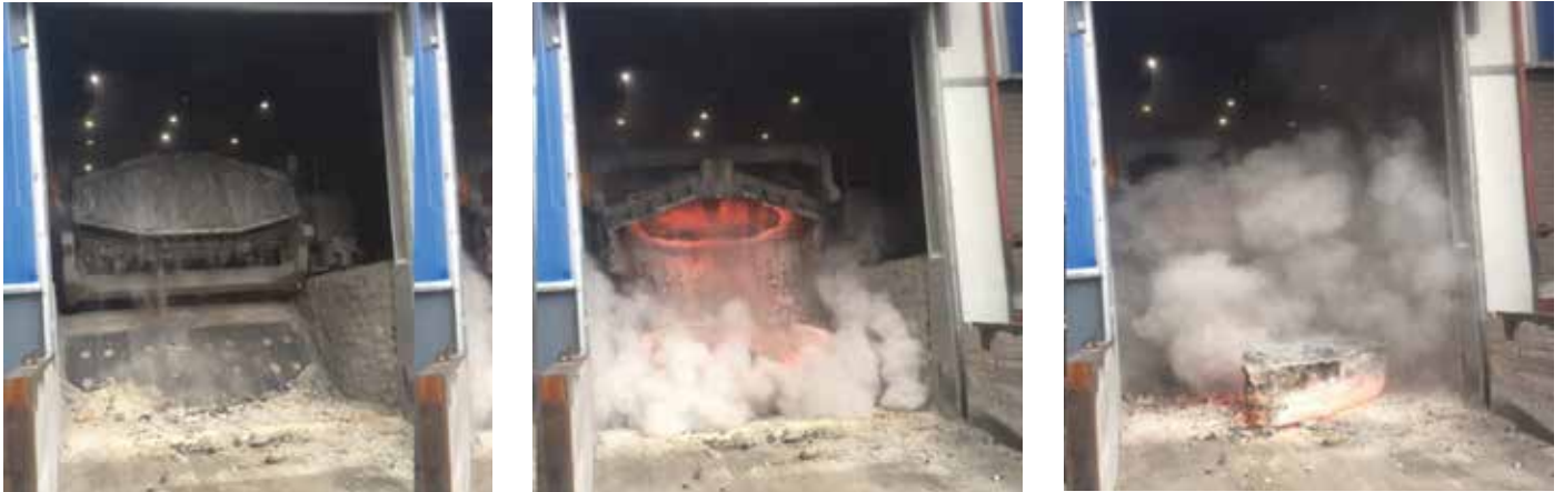
Figure 6: Tilting of the tundish and falling out of the sandwich
