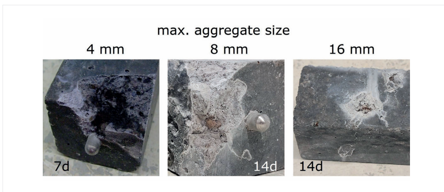
Figure 2: Damage intensities as a function of maximum aggregate size ( w/c = 0.60 ; free lime = 1.9 wt.%; test temperature = 60°C)
